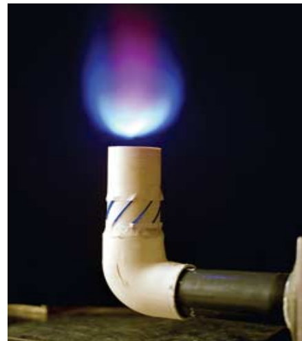
Figure 3. Low swirl burner prototype. The burner's novel flame stabilization mechanism allows it to operate at lean conditions with very
